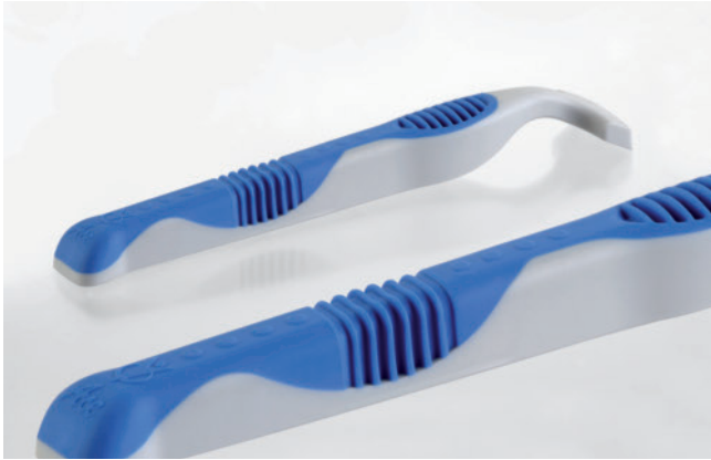
Fig. 3. The 2-component disposable razors have a polystyrene hard component and a thermoplastic elastomer for soft touch
