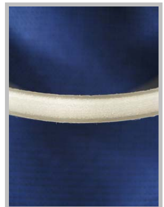
3-layer structure of a PP foamcore pipe: thin compact inner and outer layers, foamed middle layer
